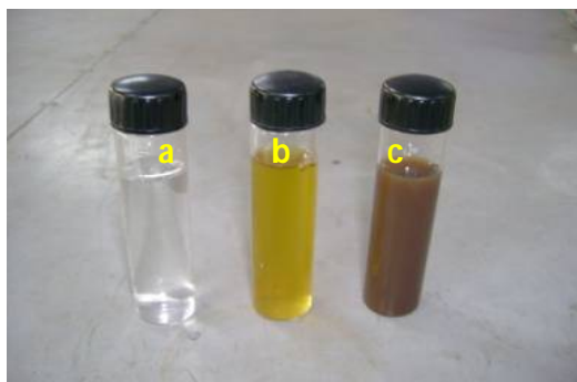
Fig 1. Optical photograph of (a) 1 mM AgNO 3 solution (b) Leaf extract (c) Leaf extract + AgNO 3 after 48 h of reaction
